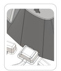
**5.** Make sure that the three edges of the magnet holder is on the outside of the assembly base
