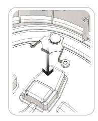
**3.** Place the magnet holder *If the toilet is connected to power, the red light goes out*
