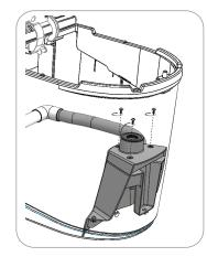
**9.** Tighten the three screws
