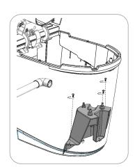
**6.** Tighten the three screws that keep the assembly base in position
