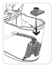
**8.** Place the fixing block and gasket
